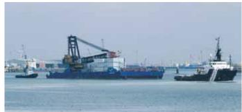
Heavy lift crane barge Conquest MB1 will install sponsons on the Costa Concordia. For this project the Conquest is outfitted with an operational 6-point mooring system from ACE and accommodation modules suitable for 60 persons from Holland Accommodation Rentals. Furthermore a full air-range diving spread has been arranged on board and the diver teams involved in the installation of the sponsons will operate from the barge.
